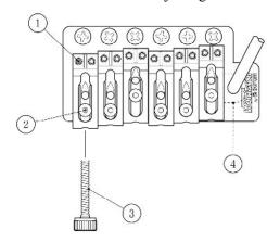
CAUTION: Ensure that you loosen the saddle-fastening screw ②, before the adjustment, or else it results in breaking down the saddle-fastening screw ② and warping the saddle and causing undesired operation.
