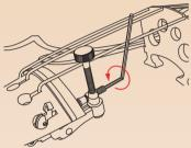
3 Making sure that the string hook moves smoothly, carefully turn the adjustment screw with a hex wrench, clamping the adjuster in place.
